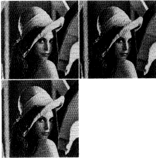
Fig. 11. Top left: original image. Top right: image reconstructed from the maxima representation shown in the second column of Fig. 9. This reconstruction is performed with 10 alternate projections, and the SNR is 28 db. Lower left: image reconstructed from the thresholded modulus maxima shown in the third column of Fig. 9 with 10 iterations on the operator P .
