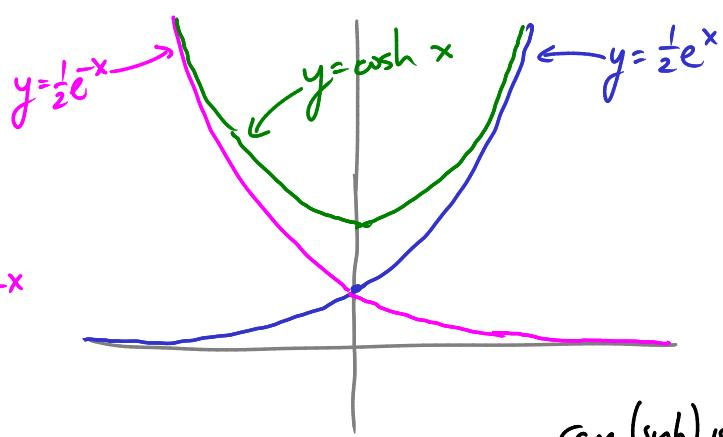
Remark:  $y = \cosh x$  is the shape of a freely-hanging heavy cord (like a telephone wire). ("catenary")
