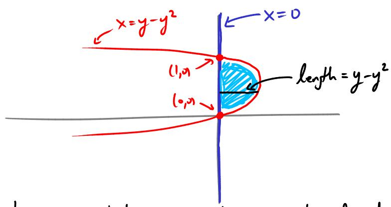
Slice by "horizontal" planes,  $y = \text{constant}$ : cross sections are circles of radius  $= y - y^2$
