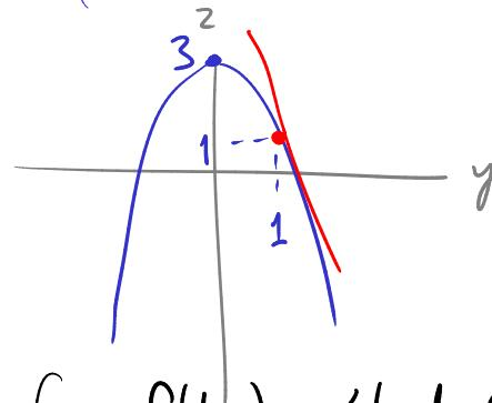
$$\begin{aligned} z &= f(1,y) = 4 - 1 - 2y^2 \\ &= 3 - 2y^2 \end{aligned}$$
