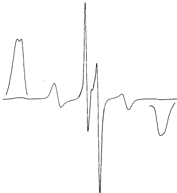
FIG. 1. Powder EPR spectrum of (\text{NH}_4)_x \text{Ti}_{1-x} \text{Al}(\text{SO}_4)_2 \cdot 12\text{H}_2\text{O} x=0.639 , 1.8% Cr, \nu=9.502 GHz, T=299 K, g=1.974 , D_1=582(2) , D_2=614(2) . The parallel features are amplified \times 40 . Separation of the low field peaks is 66 G and the entire trace spans 2900 G.
