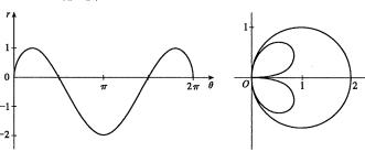
32. r increases from 0 to 1 (local max) in the interval  $\left[0, \frac{\pi}{2}\right]$ . It then decreases slightly, after which r increases to a maximum of 2 at  $\theta = \pi$ . The graph is symmetric about  $\theta = \pi$ , so the polar curve is symmetric about the polar axis.
