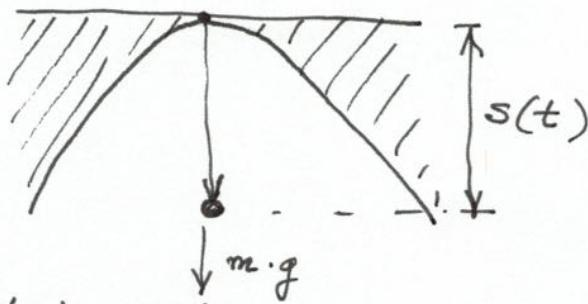
Drop stone from bridge at time  $t=0$  from  $s(0)=0$ , with velocity  $s'(0) = 1 \text{ m/sec}$ .
